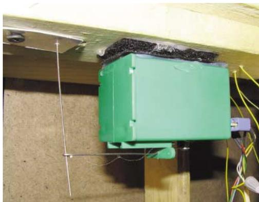
The Tortoise mounted on the bottom of the layout.
