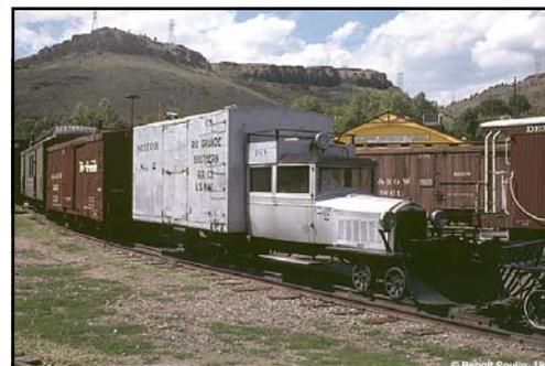
Motor #2 was rebuilt in 1939, using a 1926 Pierce-Arrow body. It was equipped with a more powerful Buick engine. Curiously, Motor #2 was placed into stand-by duty almost immediately, as other Geese were built and pressed into service. This fully-operational motor may be seen at the Colorado Railroad Museum.
